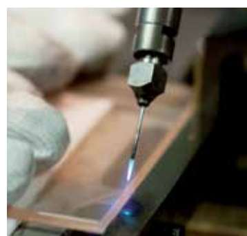
Crisp, bevelled, flame polished edges
